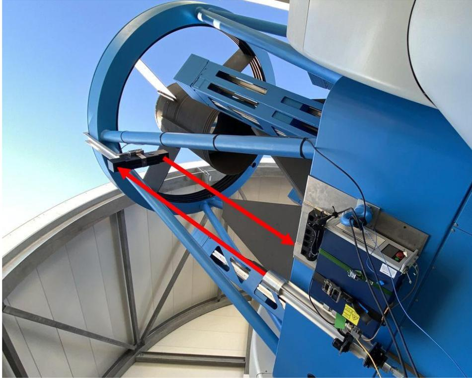
*Fig. 3: Alignment of the transmit beam pointing direction with the optical axis of the telescope. The laser beam leaving the transmit telescope and offset-reflected into the 2.3 m telescope via a retro-reflector bar is indicated with red arrows. After alignment the retro-reflector bar is rotated out of the transmit beam.*
