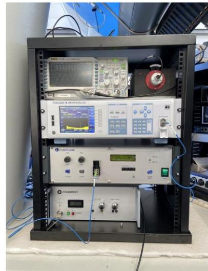
**Fig 1b:** Transmitter modulation system rack containing Coherent seed laser, Photline modulation system, Yokogawa wavemeter and Rigol oscilloscope.
