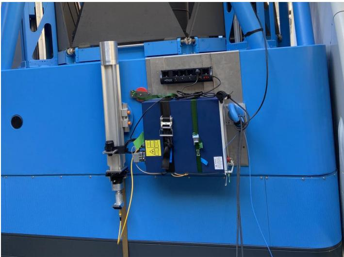
**Fig. 1a:** Transmitter telescope and optical fiber amplifier attached to the side of the main 2.3 m telescope.
