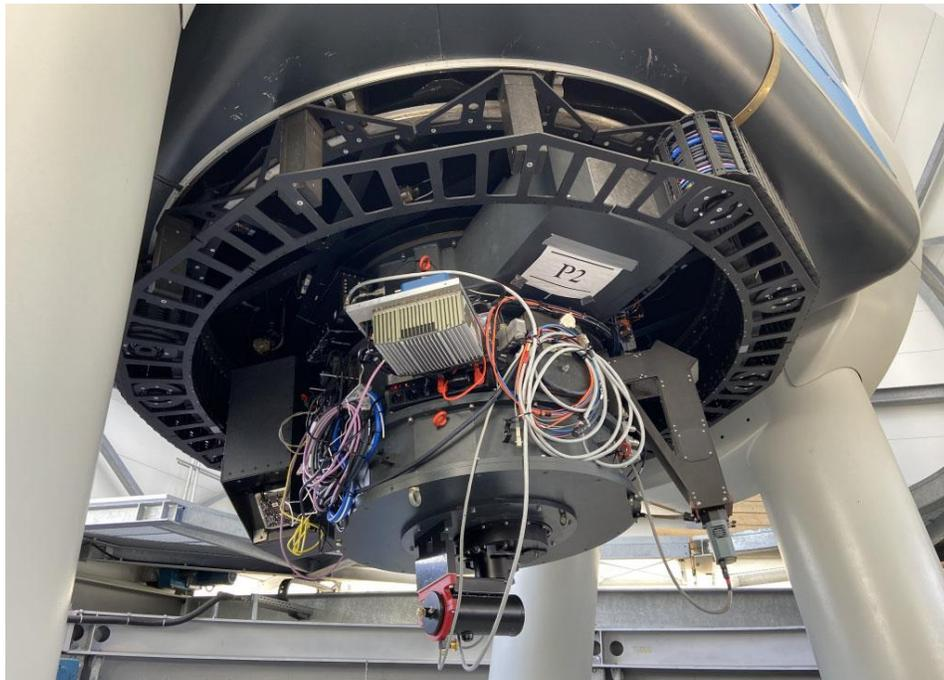
*Fig. 2: Receiver system attached to a side port of the Cassegrain focal plane. A small industrial tracking computer with silver-colored fins in the center of the image is mounted to an aluminum plate on top of which the receiver instrumentation is located.*
