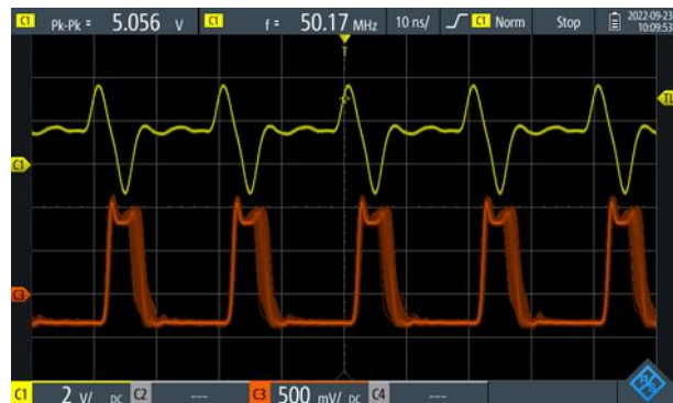
Figure 5: Delay between overdriven VCSEL and received SiPM signal
