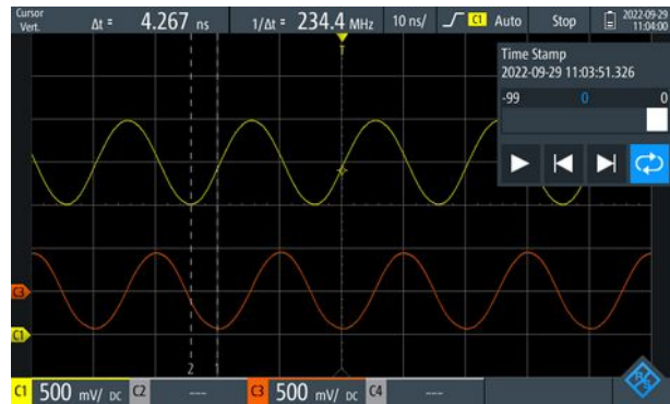
Figure 4: Phase shift between sinusoidal VCSEL driving signal and received SiPM signal
